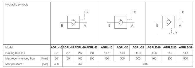
(1) Applying the pilot pressure through the pilot port X, the pilot spool opens the check valve, allowing free flow B-A.
