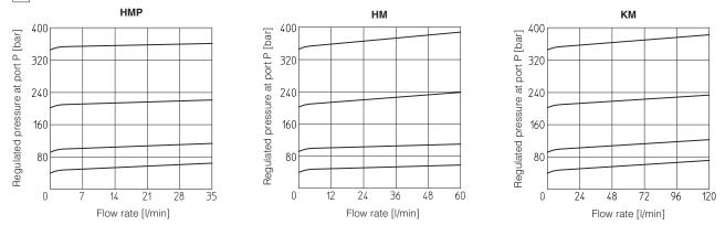
5 MINIMUM PRESSURE VERSUS FLOW DIAGRAMS (Based on fluid viscosity of 25 mm²/s at 40°C)
