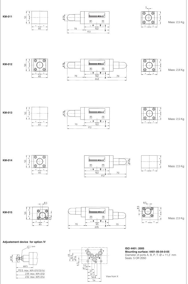
Fastening bolts: nº 4 socket head screws M6. The lenght depends on number and type of modular elements associated.
