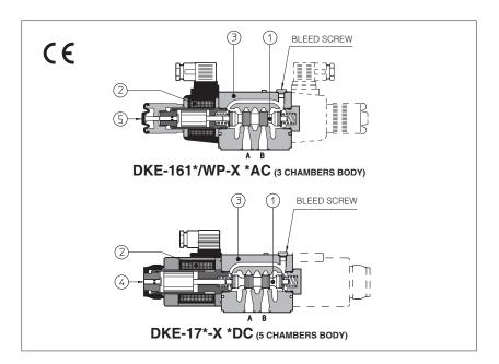
Spool type, two or three position direct operated valves with threaded solenoids certified according the North American standard cURus.
